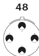
4#8 Power Service I
